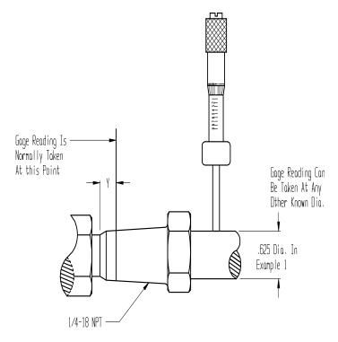
For reasons of convenience or accuracy, it may be desirable to take Micrometer Setting Gage reading from a diameter other than the recommended blank diameter at "Y". This is easily accomplished by computing a corrected gage setting dimension, using the formula:
